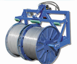
REEL UNWINDERDA: 250, 400, 500 kg and unwind spools with hydraulic brake.
